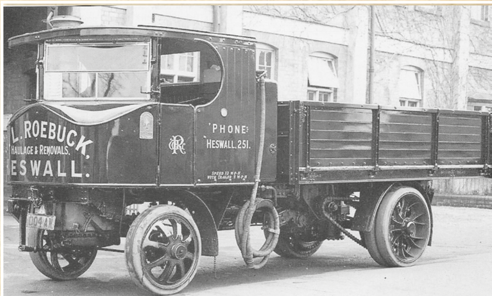
Above: 1926. This Sentinel Steam Wagon DG4 Tipper, which was built for Wm Roebuck Haulage Removals of Radmor Avenue & Pensby Road Heswall.
